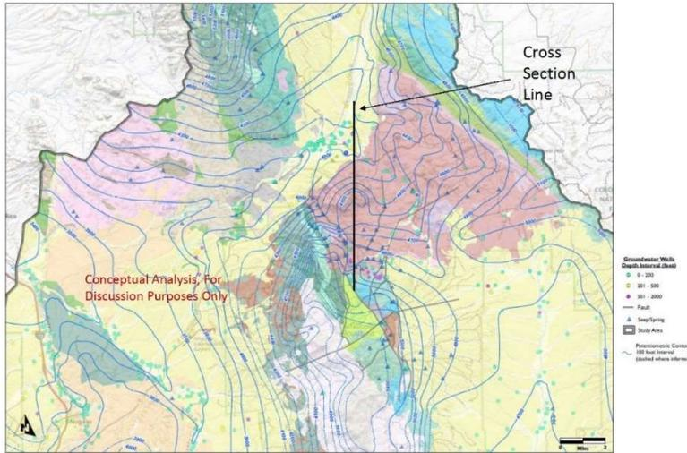
Ty: They may not be active faults, but the reason that we need to have them in a hydrologic model, is that there could be crushed material that would increase the porosity and make it easier for water to flow in that region. Or you may have an impermeable unit that has been shifted up against a more permeable unit. In that case, the fault becomes impermeable.
