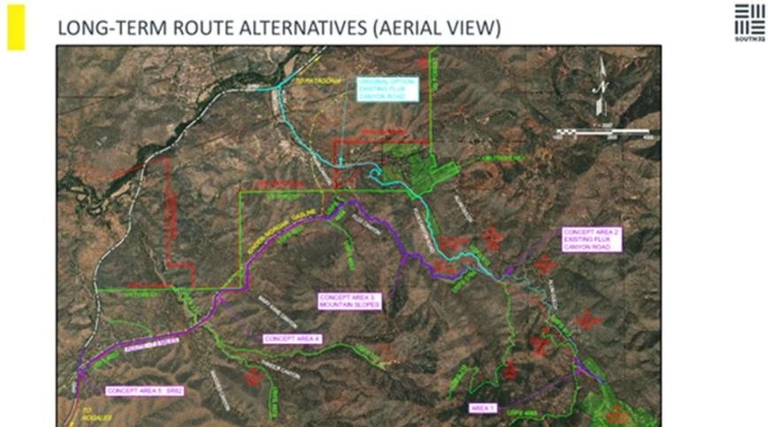
In the slide above the blue line is the Flux Canyon Road, the previously communicated long-term route preference. The new alternative is in purple which connects partly to Flux Canyon Road and closely follows the Kinder Morgan gas line and connects to SR82 further towards Nogales
