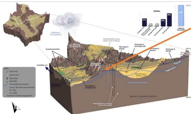
This slide [left] is a cross-section through the mountains, cutting through just south of where the South32 patented claims are [see the arrow pointing to the orange mark]. We have water that is going underground and is flowing at different depths. We have some shallow flow, we have some deeper flow, we have flow that is coming towards this region in here. We have this kind of closed area here. We have some other flow that's
