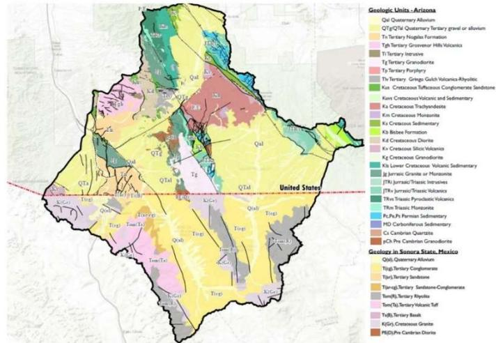
In this slide [below left] it shows that there are a lot of faults in this region which could be either conductive or restrictive to flow.
