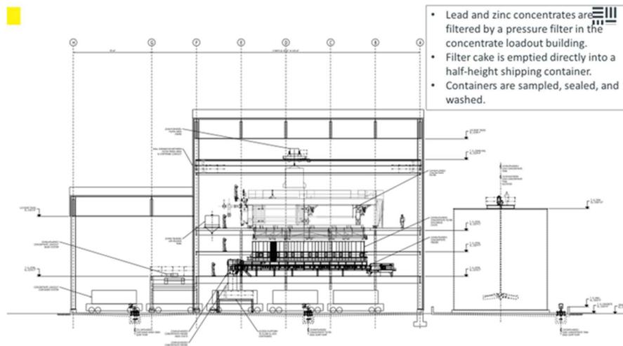
The filter cake drops straight into a half pipe container. Someone will take a product sample, to test for moisture and quality, moisture so that we ensure that it's safe for ship cargo holds. And then it is closed and sealed. Next is a truck and container wash. This is done within a covered building. All that water is blended into the sump pump on that concrete container and then goes back into the water recirculation that's used for processing.
